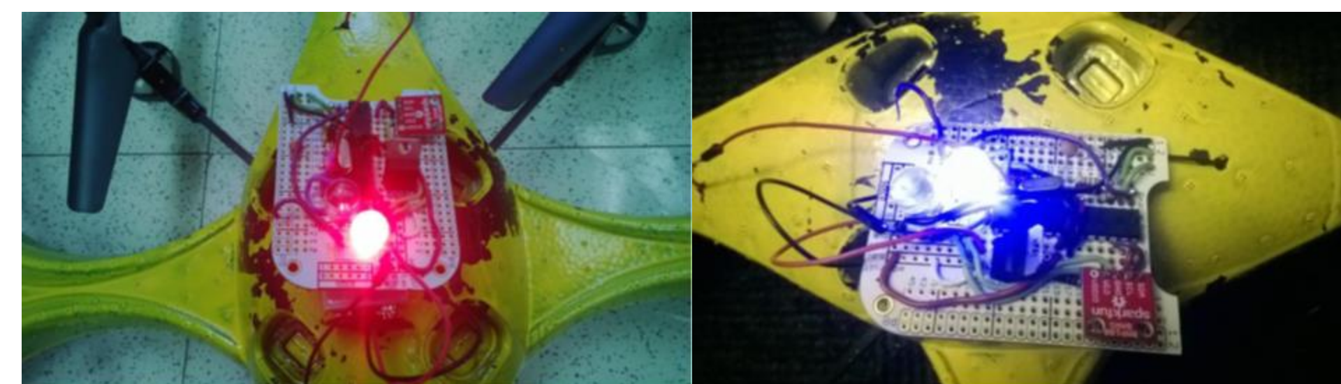
Altitude Sensing: Below 15 Feet(red) and Above 25 Feet(Blue)
