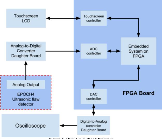
Figure 1- High Level Block Diagram
