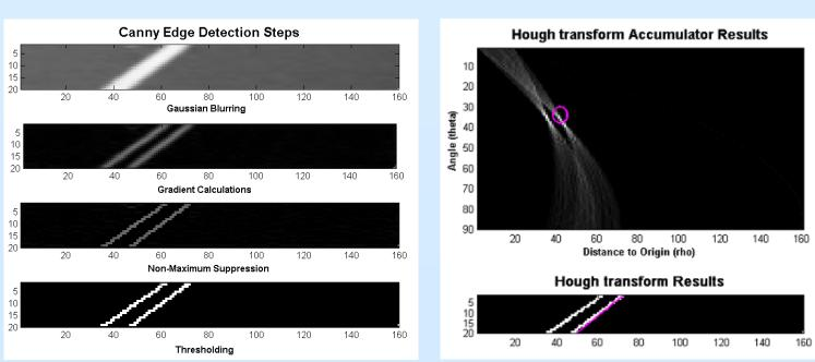
Canny/Hough Edge Detection DSP Results
