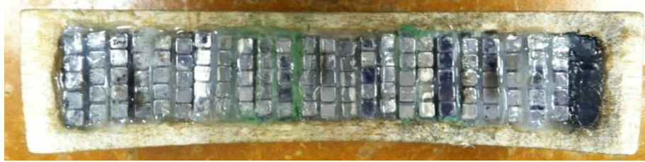
Figure 8: Halbach Array Device with Magnets Glued
