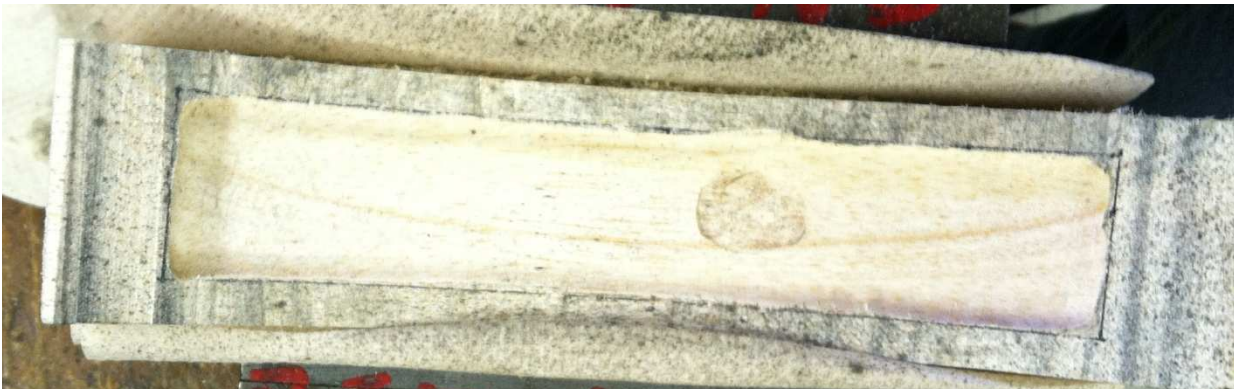
Figure 7: Balsa Wood Carved out to House Magnets
