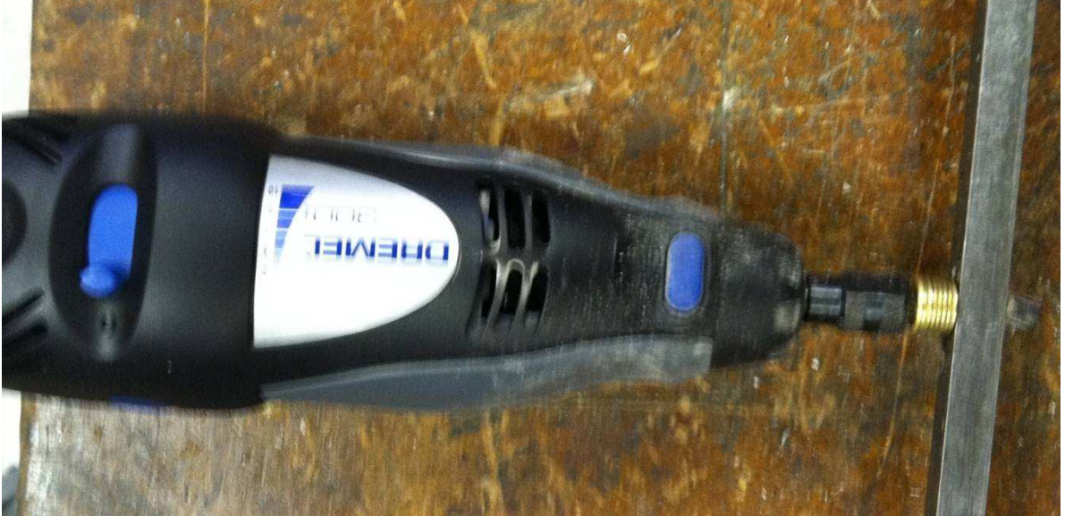
Figure 6: Dremel Setup for Carving out the Balsa Wood
