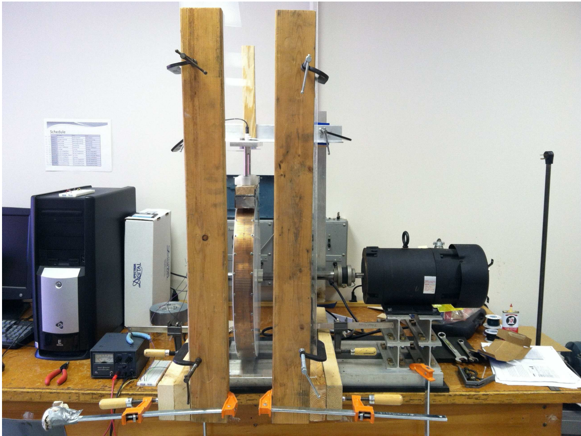
Figure 11: Experimental Set up with Shield and Displacement Sensor
