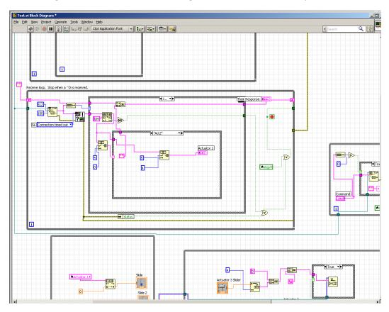
**Figure 5:** Segment of LabView Block Diagram for Client Program. Center block is a while loop for TCP read functionality
