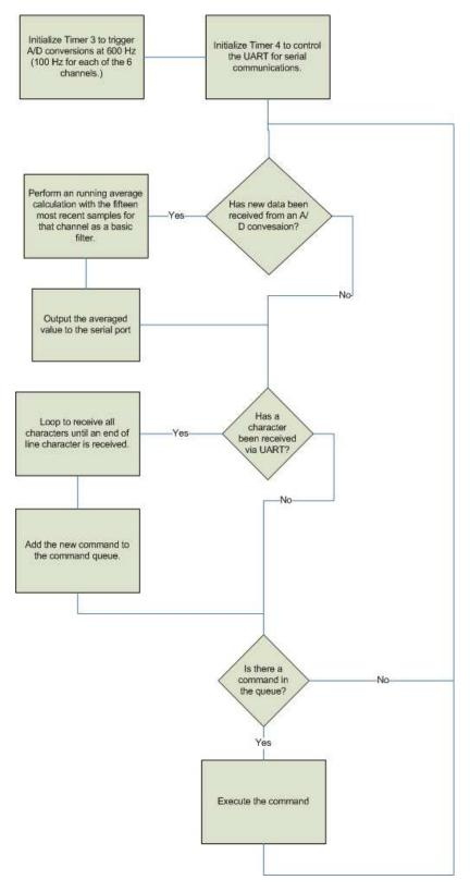
Figure 3: Overall Flowchart of Microcontroller Code
