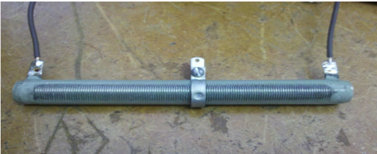
Figure 10-1, Damping Resistor 25 ohms
