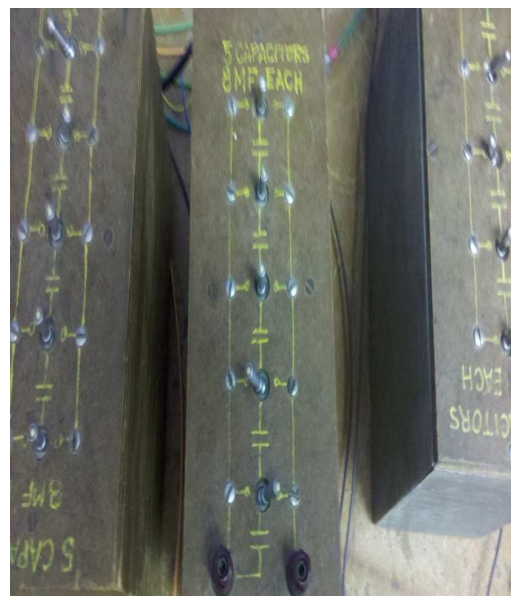
Figure 9-4, 40uF Capacitor Bank
