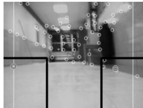
Figure 16. Corners algorithm example
