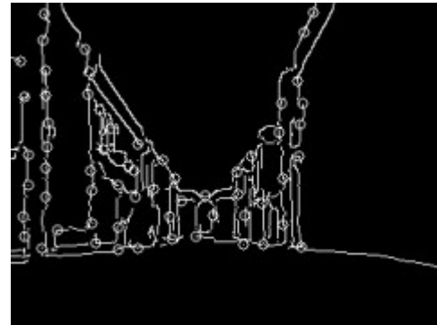
Figure 8. Corner Detection on image in Figure 7
