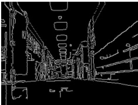
Figure 6. Edge detection on an un-blurred image
