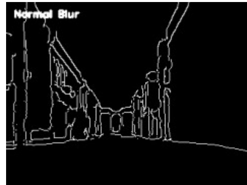
Figure 7. Edge detection on a blurred image
