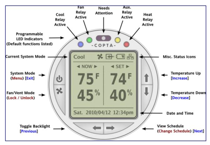
The user interface currently has 3 discrete modes. First is the "home" screen which shows the current date and time, temperature and humidity, temperature setpoint, and current operating mode. Second is the scheduling menu which shows the current schedule. Third is the settings menu which lists the memory registers and allows changes to be made to the thermostats configuration. A photo of the current "home" screen, as displayed on the prototype device, is shown below.
