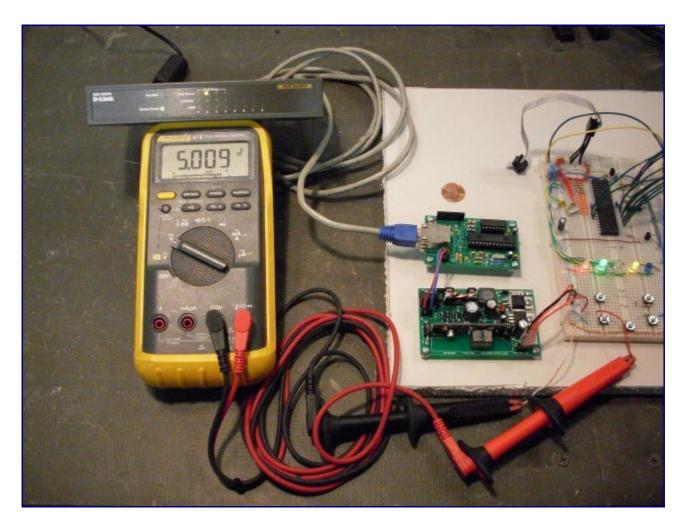
I noticed during the initial power up that the output from the PoE module was not only not 5 volts, it was much lower, being about 4.2 Volts DC. After reviewing the PoE module's datasheet as well as my schematic and PCB layout, I discovered my mistake.
