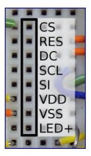
Figure 2 shows the LCD connector pinout (click thumbnail for complete view):
