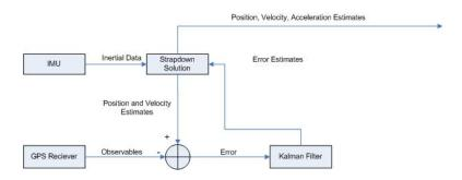
Figure 3: System Block Diagram [2]
