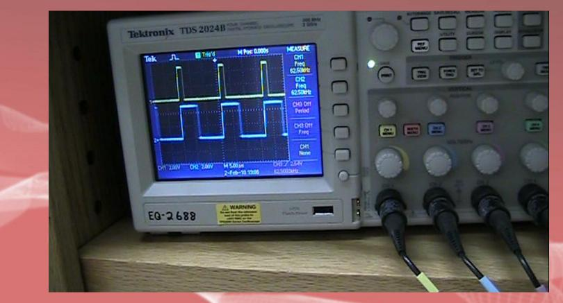
Two IR sensors independently control two PWMs.
