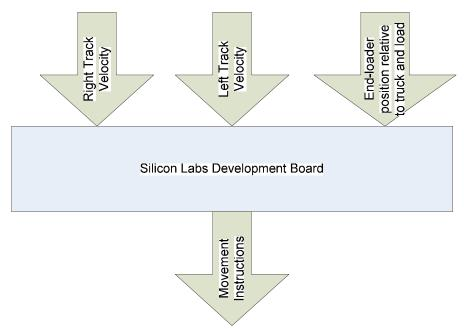
Figure 4: Development Board Subsystem Block Diagram
