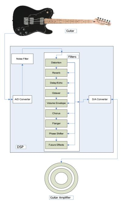
The signal comes from the guitar and goes to the DSP. It is converted to a digital signal first, then it passes through a noise filter. From the noise filter, it goes to the user-defined effects filters. After this, the modified signal is converted back to analog and is sent to the guitar amplifier for sound generation.
