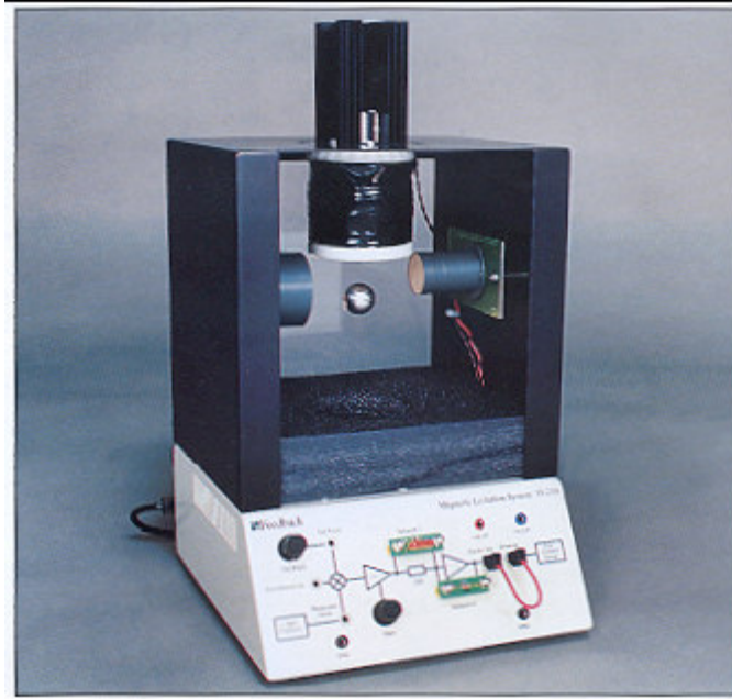
Figure 2: Photo of Magnetic Suspension Plant
