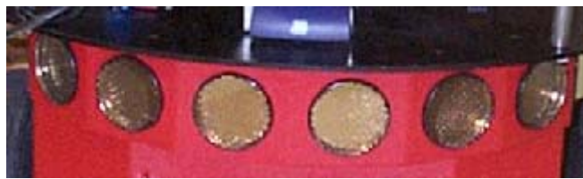
Figure 6 – Ultrasonic Sensors on the Robot
