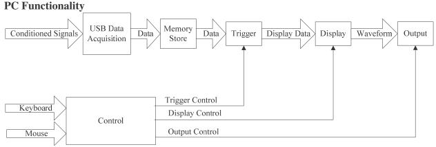
Figure 6: PC Block Diagram
