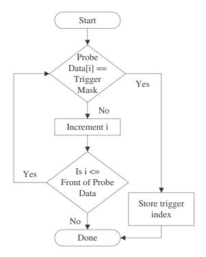
Figure 10: Trigger Block
