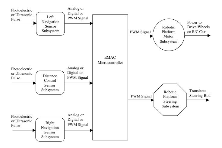
Figure 7.1 Hardware Subsystem Block Diagram
