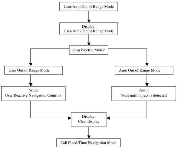
Figure 4.1 User/Auto Out of Range Software Flowchart
