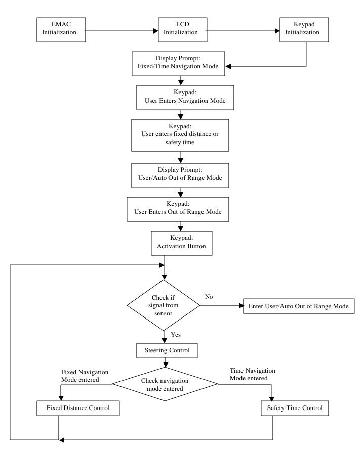
Figure 8.1 Fixed/Time Navigation Mode Software Flowchart
