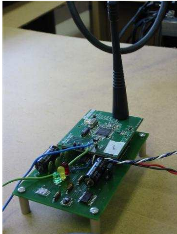
Figure 7: CC1010 Evaluation Module with WISENET Add-On Module
