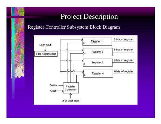
Description of Register Controller Subsystem.
