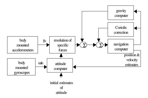
Strapdown solution in navigation frame (local North-East-Down frame) wib is the angular movement of the land vehicle fb is the acceleration of the land vehicle
