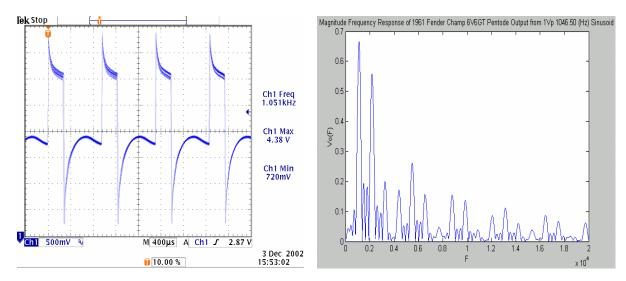
Figure 11: Output at Single-Ended Power Tube Stage of 1961 Fender Champ at Volume 12 for a 1Vp, 1046.50 (Hz) Sinusoidal Input
