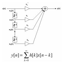
**Figure 5: FIR Digital Filter Algorithm**
