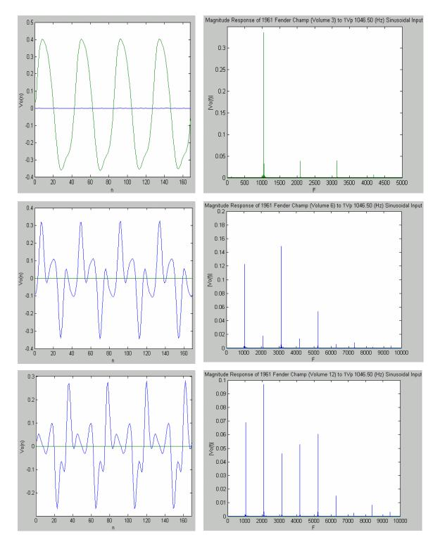
Figure 9: Fender Champ Output in 16-bit Digital Audio Data for 1Vp 1046.50 (Hz) Sinusoid at Volumes 3, 6, and 9
