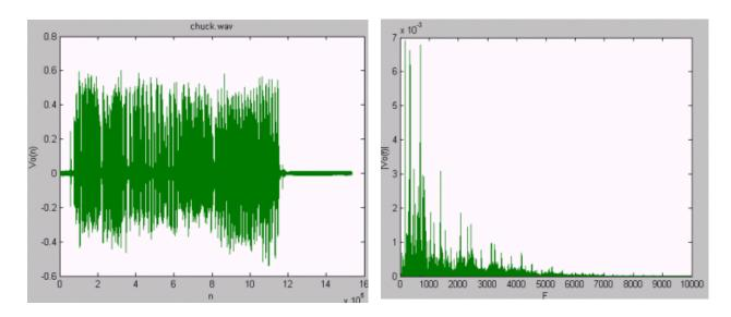
Figure 12: Fender Champ Output from a 1952 Telecaster Input
