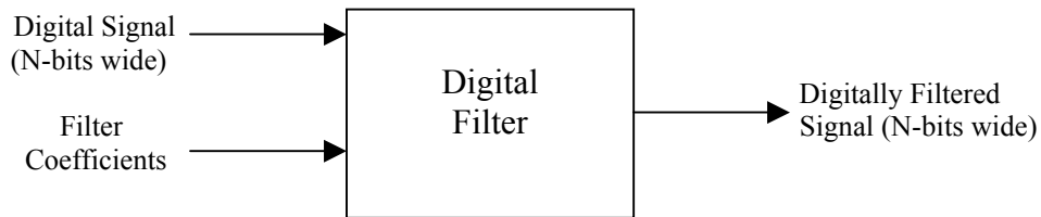
Figure 3: Block diagram of the general digital filter.
