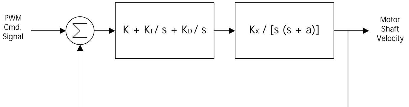
This more detailed look at the Top-Level Block Diagram of the overall system illustrates the basic forms that the block transfer functions will follow. As more detailed models of the PID Controller and DC Motor are derived, this diagram will increase in complexity. Also, a method of creating an error signal based off the Speed Command Signal and Motor Shaft Velocity Signal will need to be developed.
