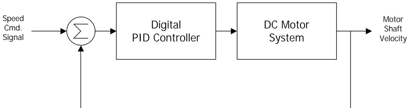
The top-level system block diagram illustrates the Digital PID Controller and DC Motor System in a closed loop configuration. The Motor Shaft Velocity will be fed back and compared with the Speed Command Signal to drive the system by means of an error signal.
