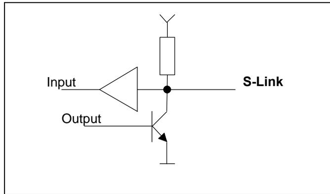
But why using 2 IO pins for input and output ? Opto couplers for isolating the S-Link from supply and other links are working unidirectional. If your PC is grounded and the CD is connected to an Amp which itself is wired to a tuner with connection to an antenna somewhere in town - then isolation might be a good idea.
