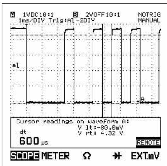
Since the delimiter between any line low state is constant, it is not necessary to detect falling and rising edges. The delay between two rising edges can be interpreted as Sync, Ones and Zeros.
