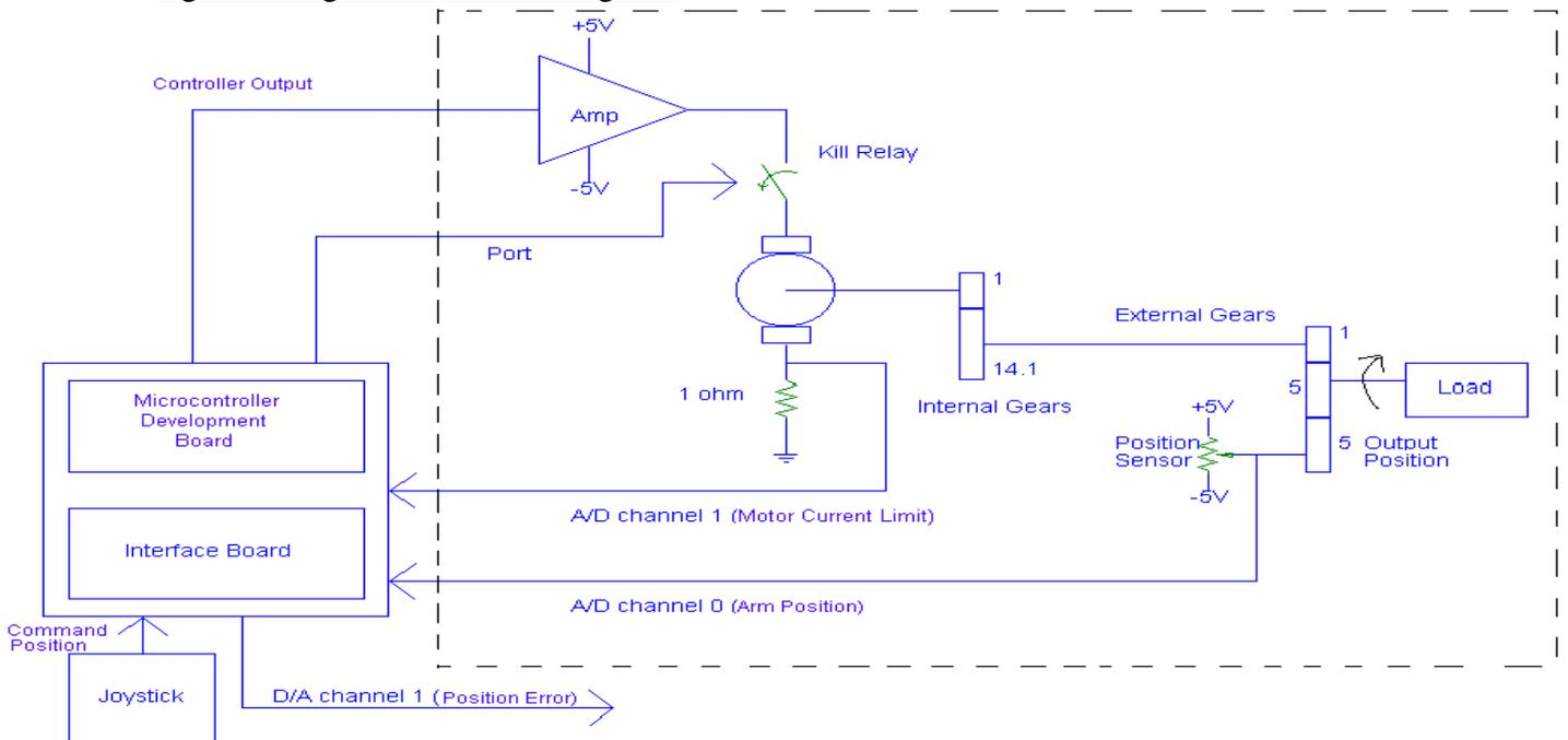
The following signals will be available on the D/A converter output channels. The expanded control block diagram is shown in Figure 3.
