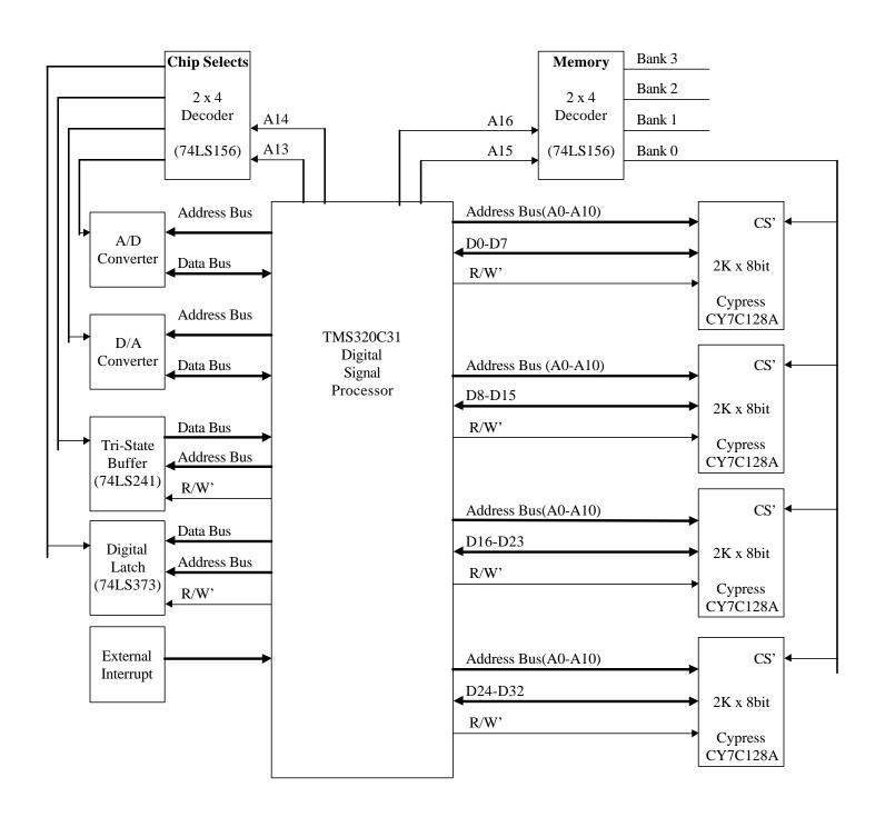
Fig.1 Block Diagram of Subsystems
